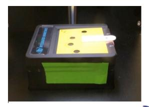
Base of **IB Fingerprint System** for application of SARS-CoV-2 stock virus solution. A LIDR-designed fingerprint template (yellow) was used to align SARS-CoV-2 stock virus solution with the platen fingerprints:
