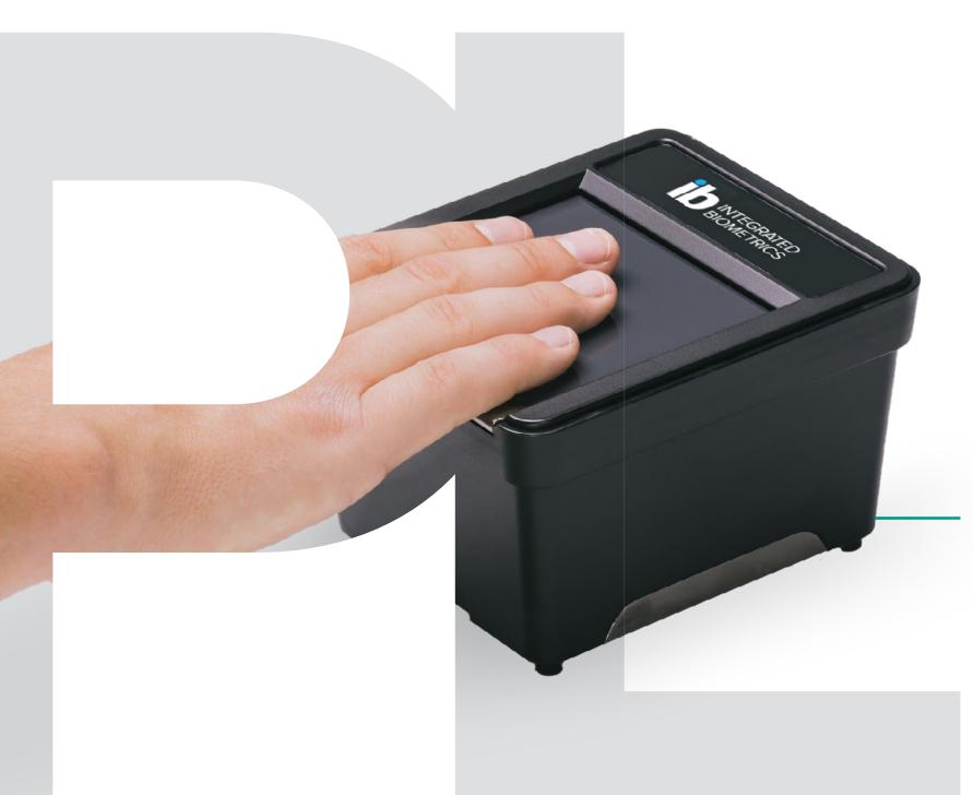
NIBSS selected IB's Kojak PL, an FBI Appendix F Certified FAP 60 10-Print roll fingerprint scanner. Small and lightweight (less than 725 grams/1.6 pounds), the Kojak PL is exceptionally robust, fast, and accurate, with a full-featured SDK that enables effective integration into applications requiring certified FAP 60 quality images.
