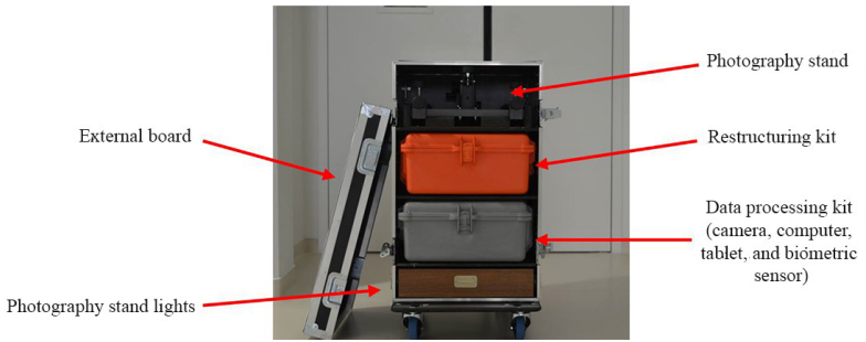
Figure 2 The different components of the Fingerprint DVI toolkit.
