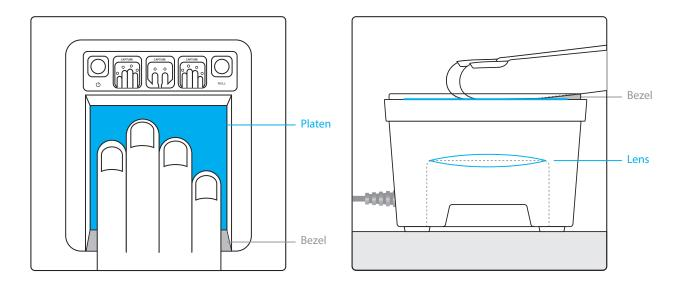
Since LES sensors rely upon conductivity from the bezel across the finger to the platen to generate an image, LES scanners automatically position fingers for optimal scanning and maximum surface area. Any attempt at spoofing using non-conductive materials is automatically rejected, since no image can result.
