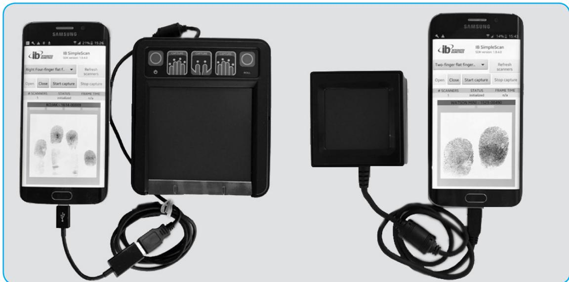
Image files transfer to host PCs, tablets or smartphones using an ordinary USB interface. This connection also acts as the sensor's power source, removing the need for a separate wired connection or battery pack. LES scanners can operate for hours using a cell phone battery without additional auxiliary power, making this technology ideal for field operations using smartphones and tablets.
